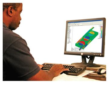
Finite element analysis software allows the modeling of complex waveguide structures.
