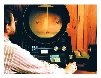
Mechanical specifications are closely inspected with an optical comparator.
